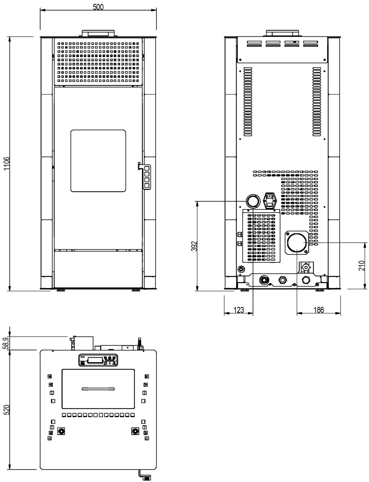
Fig. 10 - ABMESSUNGEN Idron 15 - Idron 22 - Idron 22 H2O
