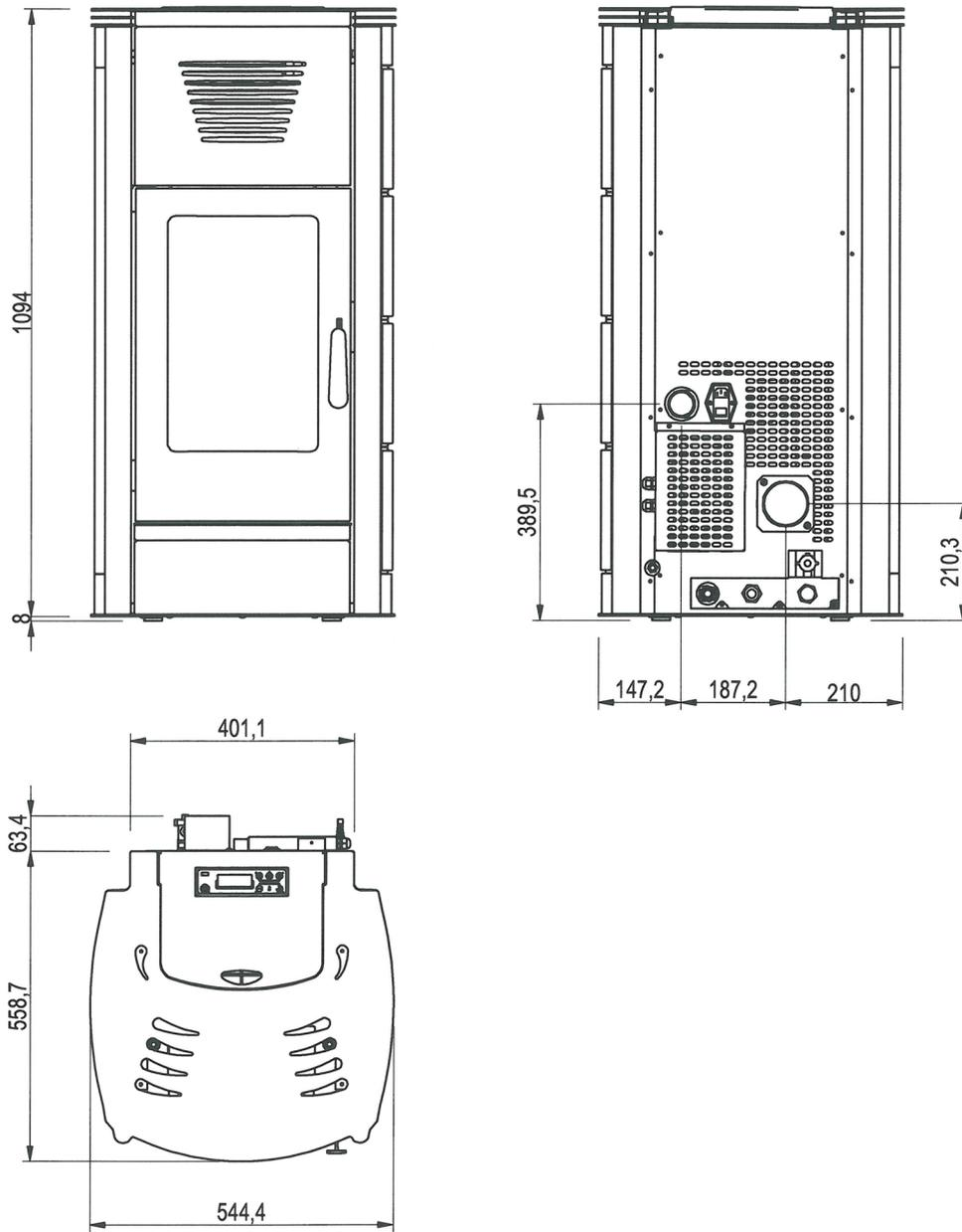
Fig. 6 - ABMESSUNGEN Aquos 15 - Aquos 22 - Aquos 22 H2O
