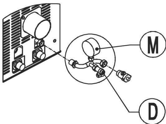
Fig. 22 - ARMATUR MIT FÜLLHAHN (D) UND MANOMETER (M)
